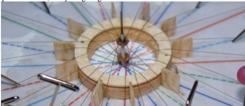
All upper spokes finished, ready for gluing
